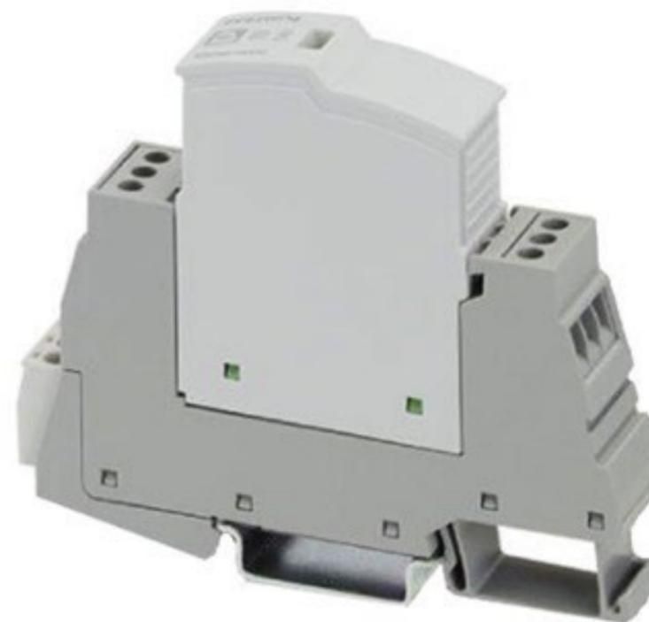
Figure 3. The Phoenix Contact 2907916 PLT-SEC Series Type 3 surge protection device with a nominal voltage rating of 24 V AC/DC (Image source: Phoenix Contact).
