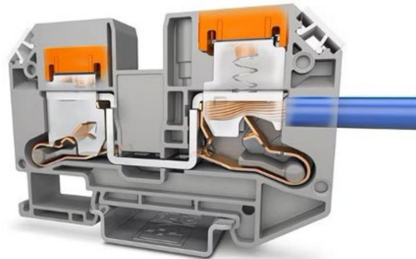
*In its factory setting, the pusher is depressed. The orange pusher pops up when the contact spring engages a conductor. (Image courtesy: Phoenix Contact.)*
