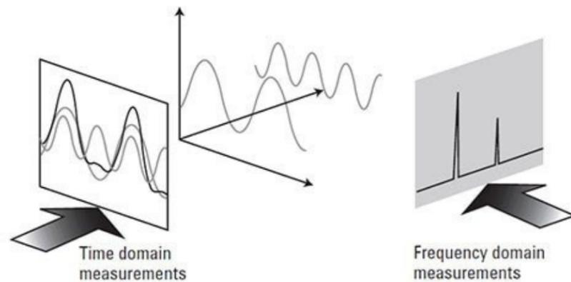
Figure 3: Relationship between a time domain signal (of which is displayed on an oscilloscope) and frequency domain signals (of which are displayed on spectrum analyzers) *Image source: Agilent Technologies [3]*
