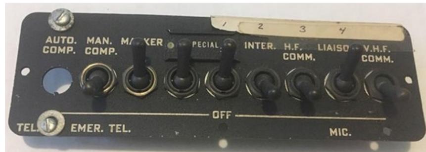
Figure 6: This array of military surplus toggle switches was used to simulate the action of limit switches on a load frame during an ongoing product development process. *Image source: Bill Schweber*
