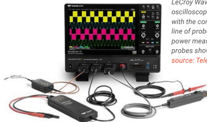
resistance ( $R_{ds}$ ) of the power FET. This requires measuring a voltage on the order of one or two volts on a waveform with a peak-to-peak swing on the order of 400 volts. The WaveSurfer 4000HD series is compatible with all Teledyne LeCroy probes compatible with the scope's bandwidth range (Figure 5).
