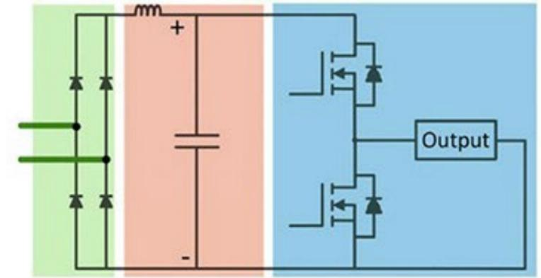
Figure 1: Shown is a functional block diagram of a switched-mode power converter for full-wave rectification of the line voltage to generate a DC bus voltage. Image source: Teledyne LeCroy
