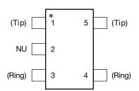
Terminal typical application names shown in parenthesis. NU - Non-usable; no external electrical connection should be made to this terminal.
