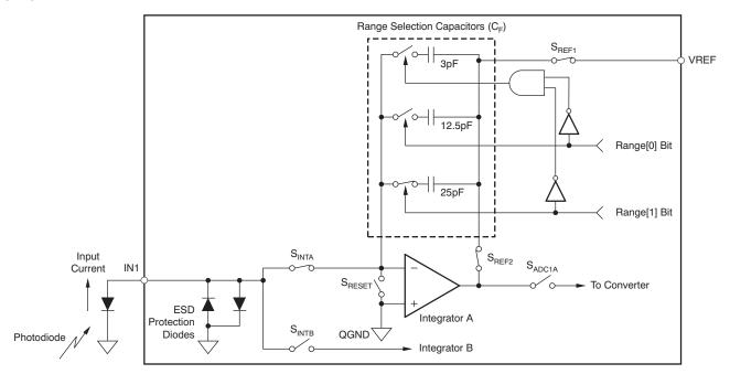
Figure 20. Basic Integration Configuration
