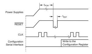
Figure 34. DDC264 Timing Diagram at Power-Up
