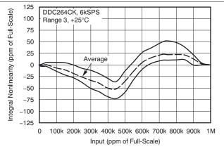
Figure 3. Integral Nonlinearity Envelope of All 64 Channels
