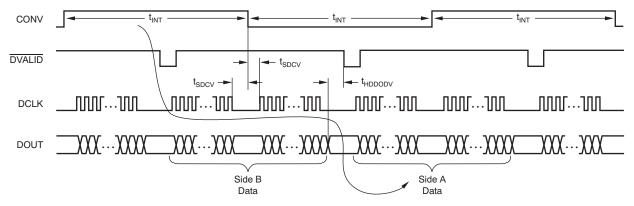
Figure 28. Readback Before and After CONV Toggles
