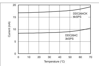
Figure 13. Analog Supply Current vs Temperature
