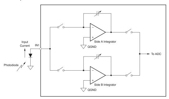
Figure 18. Dual Switched Integrator Architecture
