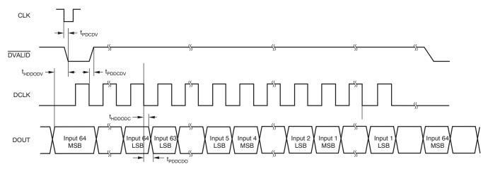
Figure 23. Digital Interface Timing Diagram for Data Retrieval From a Single DDC264
