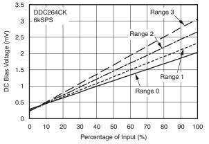
Figure 15. DC BIAS Voltage vs Input Percentage
