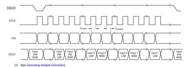
Figure 25. Timing Diagram When Using DDC264 DIN Function
