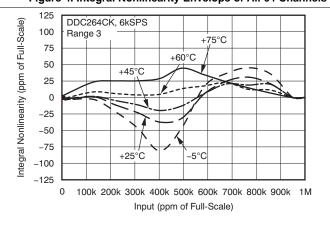
Figure 6. Integral Nonlinearity vs Temperature
