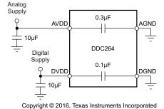
Figure 35. Power Supply Connections
