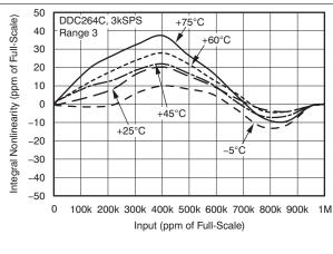
Figure 5. Integral Nonlinearity vs Temperature
