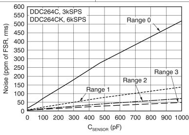
Figure 17. NOISE vs C<sub>SENSOR</sub>
