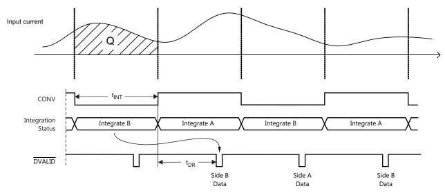
Figure 19. Integration Sequence Timing
