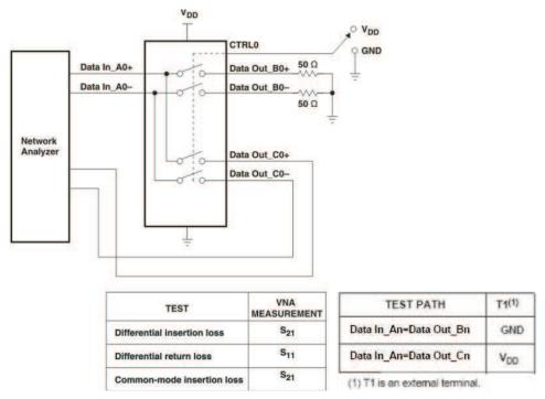
Figure 11. Differential Crosstalk Test Circuit
