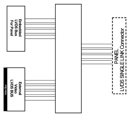
Figure 6. Typical Application for Dual LVDS
