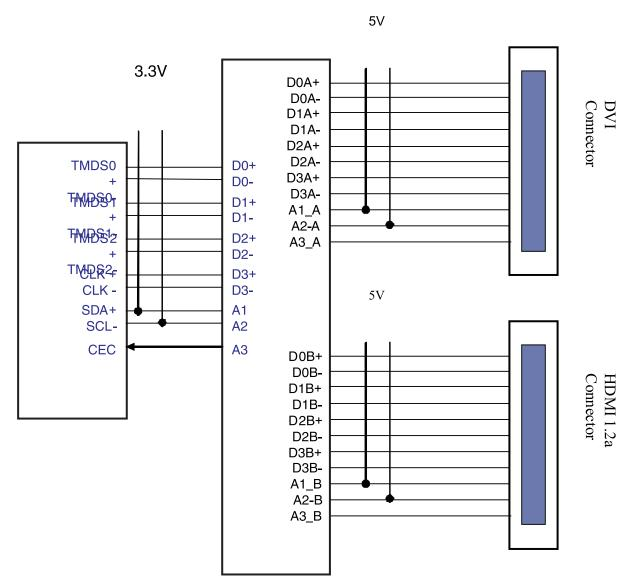
Figure 5. Typical Application Switching HDMI 1.2a and DVI
