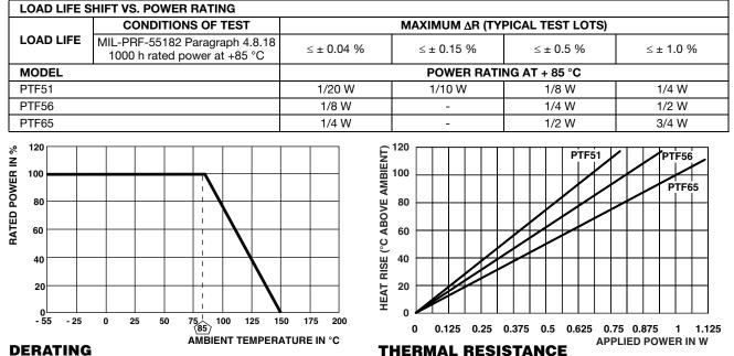
Example: When a PTF56 part is run at 1/8 W in a 70 °C ambient environment, the resistor will generate enough heat that the surface temperature of the part will reach about 17 °C over the ambient temperature, and over the life of the part this could cause the resistance value to shift up to  $\pm 0.04$  %.
