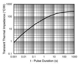
Fig. 5 - Typical Transient Thermal Impedance
