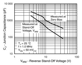
Fig. 4 - Typical Junction Capacitance
