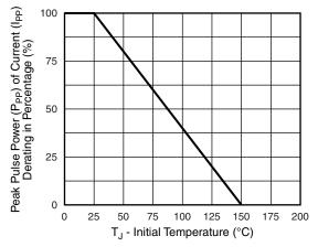
Fig. 2 - Pulse Derating Curve
