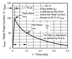
Fig. 3 - Pulse Waveform
