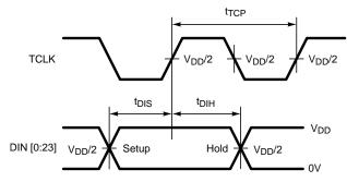
Figure 7. Serializer Setup and Hold Times
