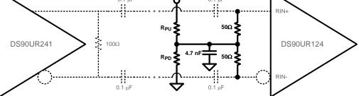
Figure 32. Receiver Termination Option 3
