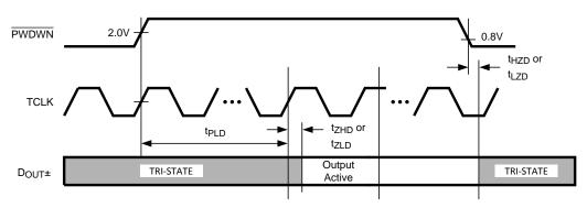
Figure 9. Serializer PLL Lock Time, and TPWDNB Tri-State Delays
