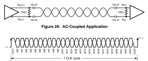
\*Note: bits [0-23] are not physically located in positions shown above since bits [0-23] are scrambled and DC Balanced
