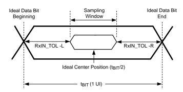
RxIN\_TOL\_L is the ideal noise margin on the left of the figure, with respect to ideal. RxIN\_TOL\_R is the ideal noise margin on the right of the figure, with respect to ideal.
