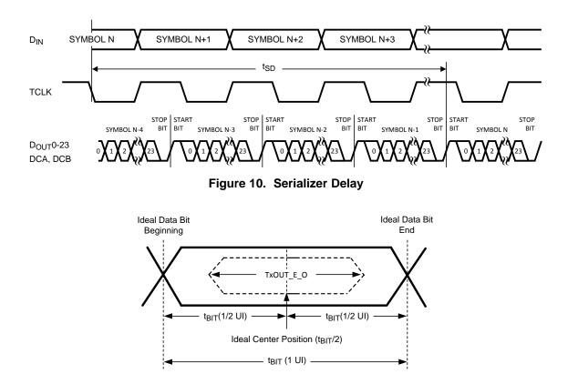
Figure 11. Transmitter Output Eye Opening (TxOUT\_E\_O)
