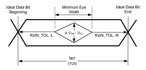
Figure 23. Receiver Input Eye Opening
