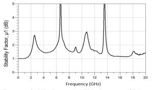
Figure 29. Stability Factor, µ1 (dB) vs Frequency (GHz) at -40 °C
