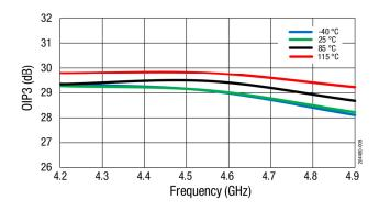
Figure 9. OIP3 (dBm) vs Frequency (GHz)
