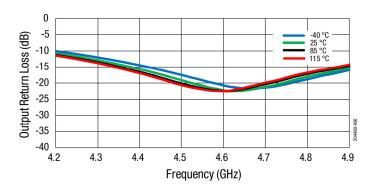
Figure 6. Output Return Loss (dB) vs Frequency
