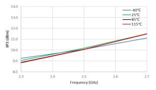
Figure 22. IIP3 (dBm) vs Frequency (GHz)
