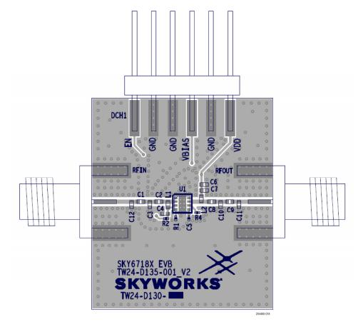
Figure 46. SKY67183-396LF EVB Assembly Diagram
