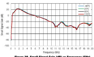
Figure 39. Small Signal Gain (dB) vs Frequency (GHz)
