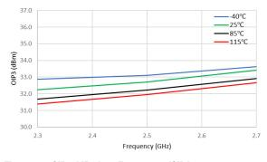
Figure 23. OIP3 (dBm) vs Frequency (GHz)
