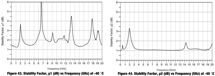
Figure 43. Stability Factor,  $\mu$ 1 (dB) vs Frequency (GHz) at -40 °C
