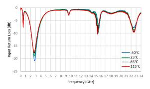
Figure 26. Input Return Loss (dB) vs Frequency (GHz)
