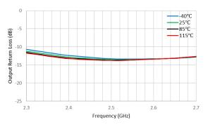
Figure 20. Output Return Loss (dB) vs Frequency
