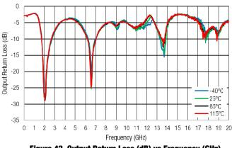
Figure 42. Output Return Loss (dB) vs Frequency (GHz)
