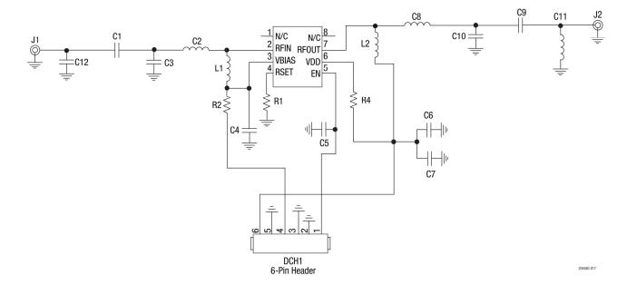
Figure 45. SKY67183-396LF Evaluation Board Schematic
