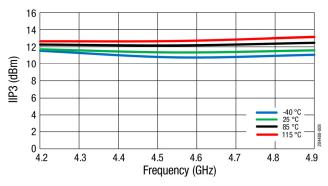
Figure 8. IIP3 (dBm) vs Frequency (GHz)
