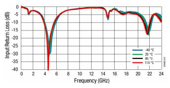
Figure 12. Input Return Loss (dB) vs Frequency (GHz)
