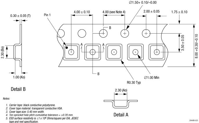
6. Ao and Bo measurement point to be 0.30 mm from bottom pocket.
