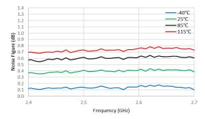
Figure 18. Noise Figure (dB) vs Frequency (GHz)
