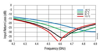
Figure 5. Input Return Loss (dB) vs Frequency
