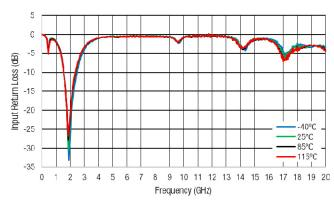
Figure 40. Input Return Loss (dB) vs Frequency (GHz)
