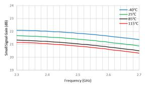
Figure 17. Small Signal Gain (dB) vs Frequency (GHz)
