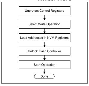
In the Flash write procedure (see Table 14-1), the Row Programming method is used to program the Flash memory, as it is typically the most expedient. word and Quad Word programming methods are also available, depending on the device, and may be used or required depending on your application. Refer to the "Flash Program Memory" chapter in the specific device data sheet and the related section of the "PIC32 Family Reference Manual" for more information.
