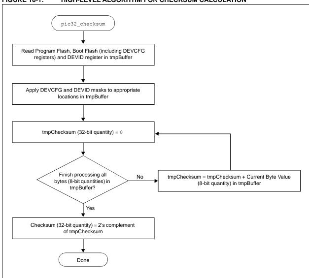
The formula to calculate the checksum for a PIC32 device is provided in Equation 18-1.
