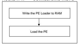
Loading the PE in the memory is a two step process:
