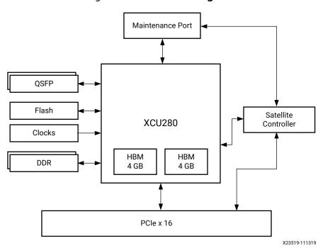
Figure 1: U280 Block Diagram
