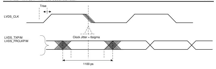
Figure 8-8. Timing Parameters
