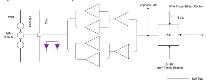
Figure 9-3. Transmit Subsystem (Per Channel)
