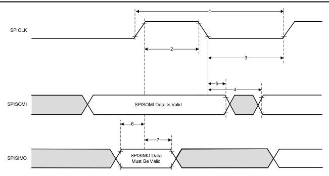
Figure 8-5. SPI Peripheral Mode External Timing
