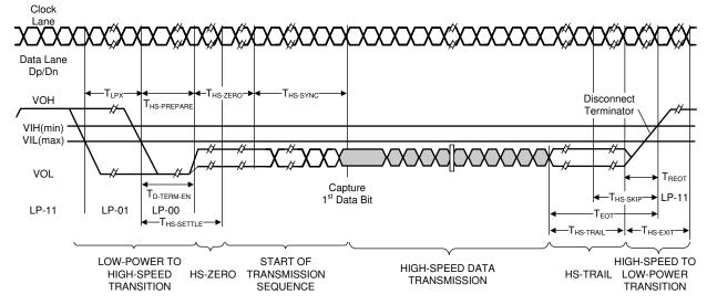
Figure 8-10. High-Speed Data Transmission Burst
