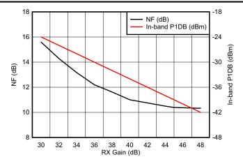
Figure 8-1. Noise Figure, In-band P1dB vs Receiver Gain
