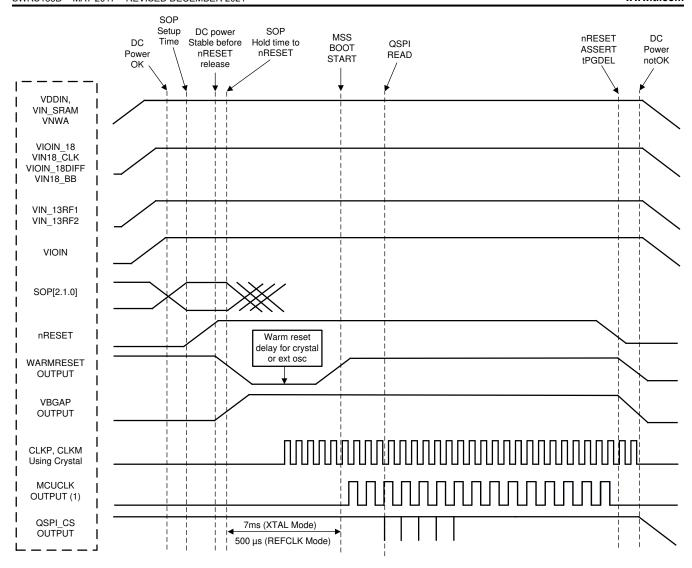
Figure 8-2. Device Wake-up Sequence
