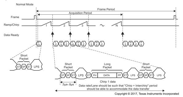
Frame Start - CSi2 VSYNC Start Short PacketLine Start - CSI2 HSYNC Start Short PacketLine End - CSI2 HSYNC End Short PacketFrame End - CSi2 VSYNC End Short Packet
