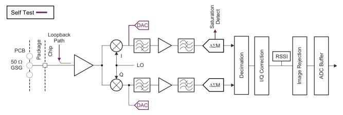
Figure 9-4. Receive Subsystem (Per Channel)
