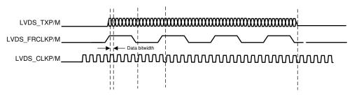
Figure 8-7. LVDS Interface Lane Configuration And Relative Timings
