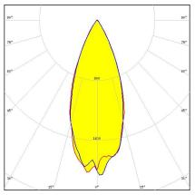
Dimensions: 9.9 mm x 9.9 mm Height: 7.00 mm ~35° wide beam with location pin installation
