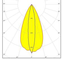
Dimensions: 10.0 mm x 10.0 mm Height: 7.90 mm ~18° x 50° oval beam with location pin
