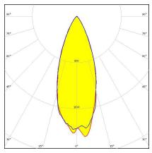
Dimensions: 9.9 mm x 9.9 mm Height: 7.00 mm ~45° wide beam with location pin installation
