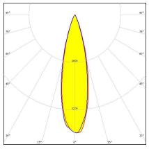
Dimensions: 10.0 mm x 10.0 mm Height: 7.90 mm ~25° medium beam with location pin installation
