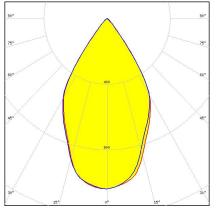
Dimensions: 110.0 mm x 110.0 mm Height: 57.30 mm ~60° wide beam. Clean appearance with no additional attachment interface.
