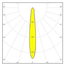
Dimensions: 110.0 mm x 110.0 mm Height: 57.30 mm ~10° spot beam
