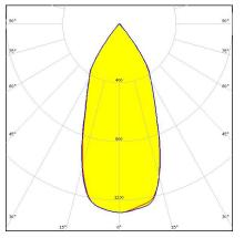
Dimensions: 110.0 mm x 110.0 mm Height: 57.30 mm ~50° medium beam. Clean appearance with no additional attachment interface.
