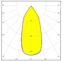
Dimensions: 110.0 mm x 110.0 mm Height: 57.30 mm ~50° medium beam
