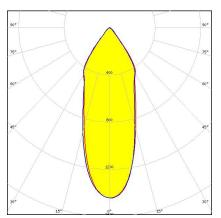
Dimensions: 110.0 mm x 110.0 mm Height: 57.30 mm ~35° medium beam. Clean appearance with no additional attachment interface
