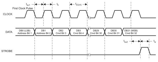
Figure 1. Serial Programming Timing
