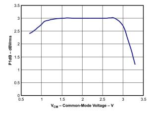
Figure 36. P1dB Performance vs Common-Mode Voltage
