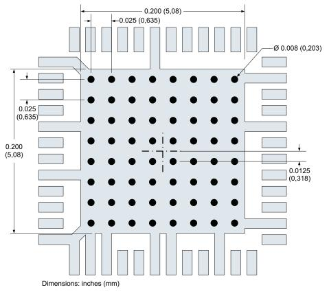
Figure 34. PCB Layout Guidelines
