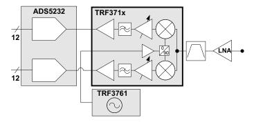
Figure 37. Block Diagram of Direct Downconverting Receiver
