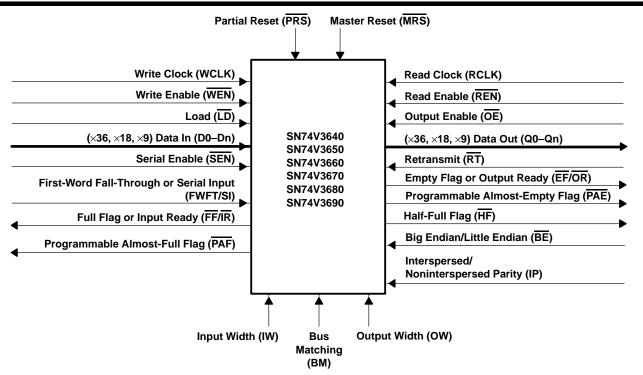
Figure 1. Single-Device-Configuration Signal Flow
