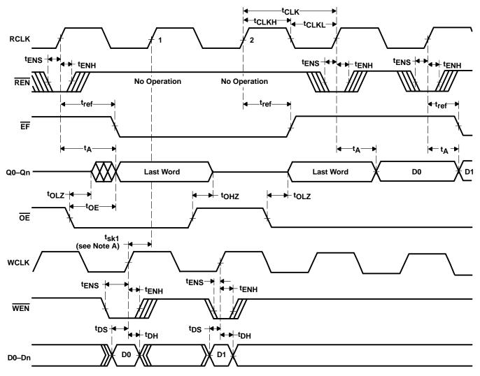
NOTES: A. t<sub>sk1</sub> is the minimum time between a rising WCLK edge and a rising RCLK edge to ensure that  $\overline{\text{EF}}$  goes high (after one RCLK cycle + t<sub>ref</sub>). If the time between the rising edge of WCLK and the rising edge of RCLK is less than t<sub>sk1</sub>,  $\overline{\text{EF}}$  deassertion can be delayed one additional RCLK cycle.
