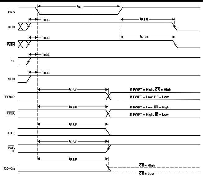
Figure 3. Partial Reset Timing
