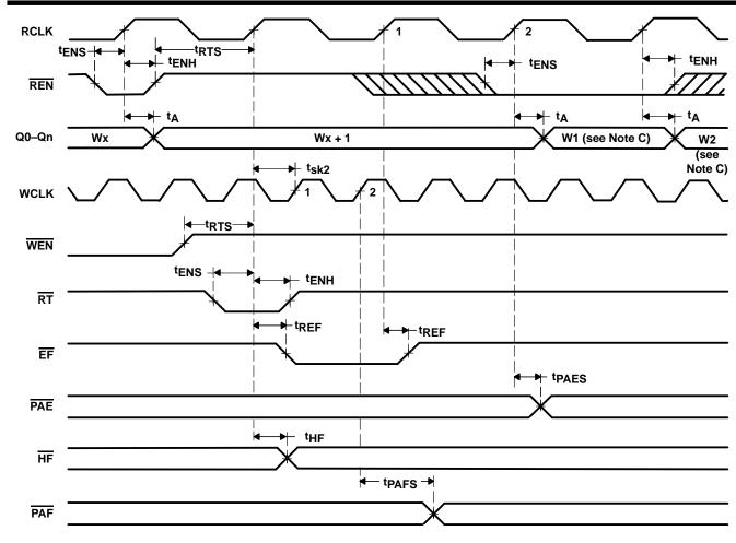
NOTES: A. Retransmit setup is complete after EF returns high; only then can a read operation begin.
