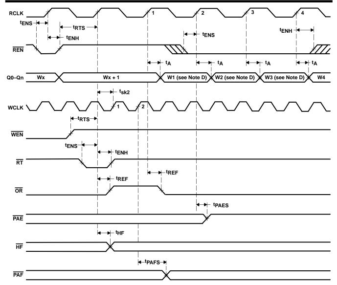
NOTES: A. Retransmit setup is complete after OR returns low.
