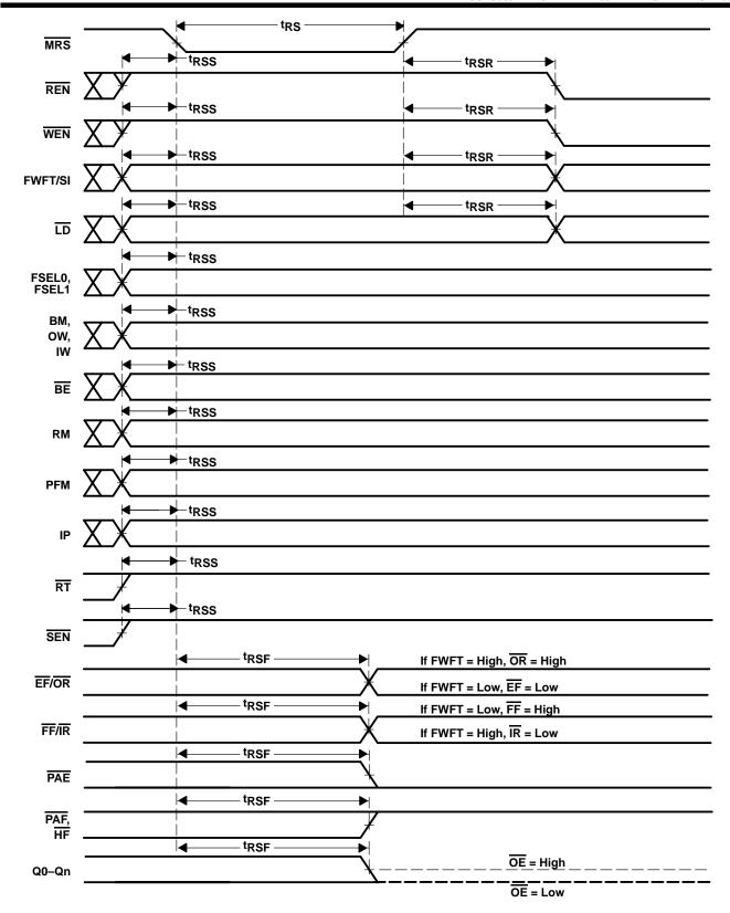
**Figure 2. Master Reset Timing**
