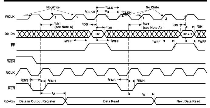
NOTES: A. t<sub>sk1</sub> is the minimum time between a rising RCLK edge and a rising WCLK edge to ensure that  $\overline{\text{FF}}$  goes high (after one WCLK cycle + t<sub>WFF</sub>). If the time between the rising edge of the RCLK and the rising edge of the WCLK is less than t<sub>sk1</sub>,  $\overline{\text{FF}}$  deassertion can be delayed one additional WCLK cycle.
