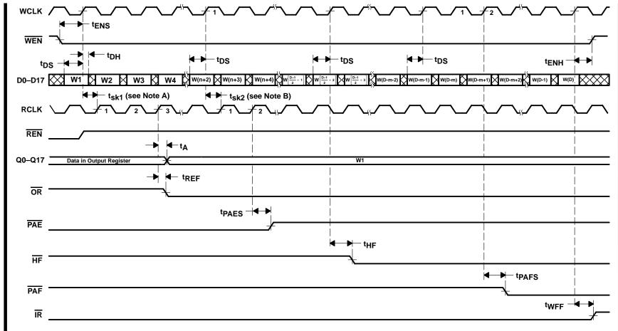
NOTES: A. t<sub>sk1</sub> is the minimum time between a rising WCLK edge and a rising RCLK edge to ensure that  $\overline{\text{OR}}$  goes low after two RCLK cycles + t<sub>REF</sub>. If the time between the rising edge of WLCK and the rising edge of RCLK is less than t<sub>sk1</sub>,  $\overline{\text{OR}}$  assertion can be delayed one additional RCLK cycle.
