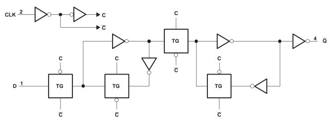
Figure 4. Logic Diagram (Positive Logic)
