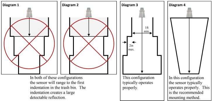
As the bin increases in size, the less likely the installation is going to detect unwanted objects and noise.
