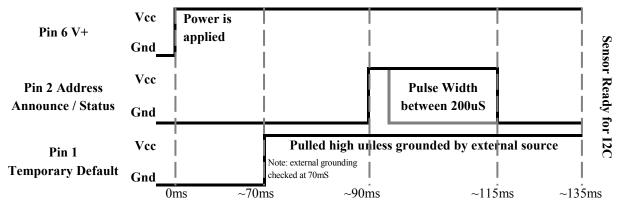
After the sensor is commanded to take a range reading it sends an ultrasonic pulse, waits between  $\sim$ 15ms to  $\sim$ 70ms to detect a target, and determines the range Then the sensor will resume I2C communications. If the sensor is addressed while in the middle of a range reading, all requests for communication will be responded with a NACK (not acknowledge).
