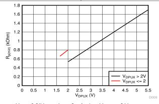
$V_{OL}$  = 0.2\* $V_{DPUX}$ ,  $I_{OL}$  = 2 mA when  $V_{DPUX} \le 2$  V  $V_{OL}$  = 0.4 V,  $I_{OL}$  = 3 mA when  $V_{DPUX} > 2$  V
