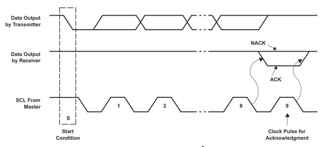
Figure 8-3. Acknowledgment on I<sup>2</sup>C Bus
