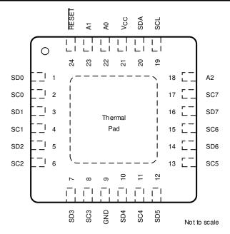
Figure 5-2. RGE Package, 24-Pin VQFN, Top View
