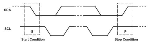
Figure 8-1. Definition of Start and Stop Conditions
