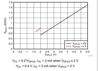
Figure 6-2. Minimum Pull-Up Resistance  $(R_{p(min)})$  vs Pull-Up Reference Voltage  $(V_{DPUX})$
