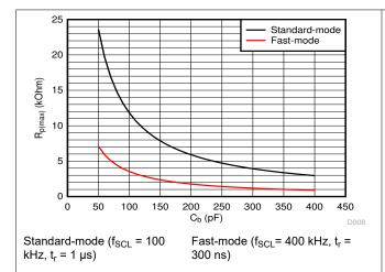
Figure 6-1. Maximum Pull-Up Resistance ( $R_{p(max)}$ ) vs Bus Capacitance ( $C_b$ )
