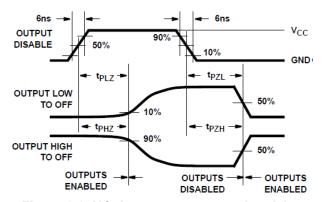
Figure 6-3. HC three-state propagation delay waveform
