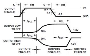
Figure 6-4. HCT three-state propagation delay waveform
