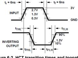
Figure 6-2. HCT transition times and tpopationg delay times, combination logic
