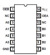
J, N, or D Package 14-Pin CDIP, PDIP, or SOIC Top View
