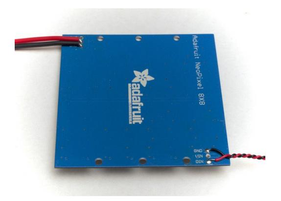
The other end of this wire pair connects to channel Zero on the Fadecandy Controller. The GND wire needs to connect to the - terminal on the Fadecandy, and the DIN wire connects to +. There are tiny + and - labels on the board, or you can remember that the pins nearest to the edge are all -.
