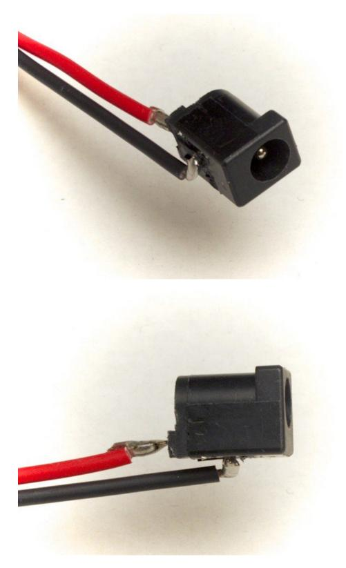
The barrel jack is almost ready to use! You'll want to insulate it, though, so you don't have to worry about metal objects bridging the two power terminals. It's especially important to watch out for short circuits when you're using such a large power supply!
