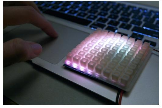
Individually addressable LEDs are everywhere. In the quest for a smaller, cheaper, smarter LED, the latest and hottest technology is the NeoPixel (https://adafru.it/cVZ), AdaFruit's term for the WS2812. This is an amazing little chip that integrates red, green, and blue LEDs with a controller chip into a single package.
