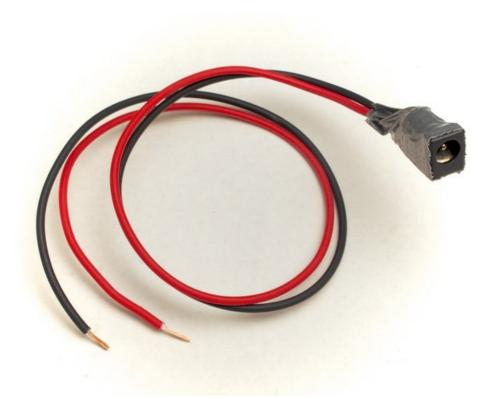
These wires will go to the VDD and GND pins on the NeoMatrix. Since we'll need a GND pin for the Fadecandy board too, it's convenient to attach these wires to the side of the NeoMatrix with DOUT instead of DIN.
