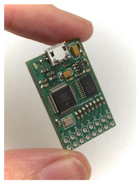
This is the component side of the Fadecandy Controller. At the top, you'll see a Micro USB connector. This is how Fadecandy gets data from your computer, and how it powers itself. The LEDs themselves draw so much power that they need a separate power brick, but the controller board requires very little power.
