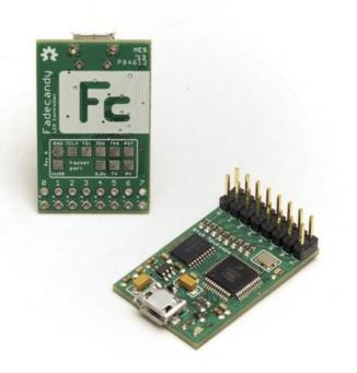
Fadecandy works with any WS2811 or WS2812 LEDs, and you can program your LEDs using many different environments. This tutorial covers one particular LED module and one particular programming environment. We'll be programming an 8x8 NeoMatrix (http://adafru.it/1487) in the Processing (https://adafru.it/cV8) language.
