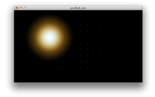
The large orange glowing dot follows your mouse. Each of the tiny single-pixel dots represents one of your 64 LEDs. With Fadecandy's Processing library, it's easy to create effects that draw to the screen and sample specific on-screen pixels for each LED.
