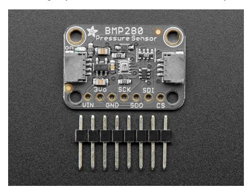
The BMP280 is the next-generation of sensors from Bosch, and is the upgrade to the BMP085/BMP180/BMP183 - with a low altitude noise of 0.25m and the same fast conversion time. It has the same specifications, but can use either I2C or SPI. For simple easy wiring, go with I2C. If you want to connect a bunch of sensors without worrying about I2C address collisions, go with SPI.
