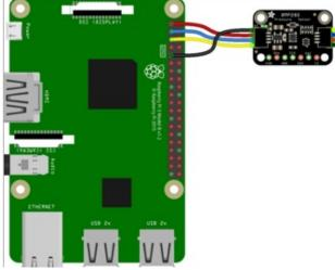
And an example on the Raspberry Pi 3 Model B wired with SPI:
