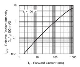
Fig. 5 - Relative Radiant Intensity vs. Forward Current
