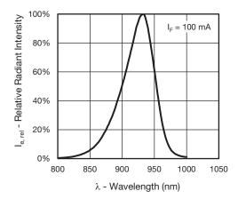
Fig. 7 - Relative Radiant Intensity vs. Wavelength
