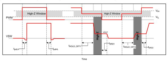
Figure 2. PWM Tri-State Timing Diagram
