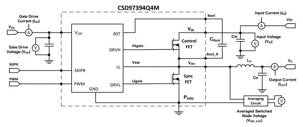
Figure 15. Power Loss Test Circuit
