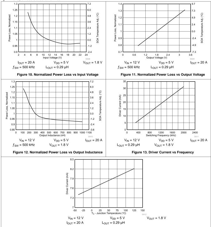
1. The Typical CSD97394Q4M System Characteristic curves are based on measurements made on a PCB design with dimensions of 4.0 inches (W) x 3.5 inches (L) x 0.062 inch (T) and 6 copper layers of 1 oz. copper thickness. See the *System Example* section for detailed explanation.
