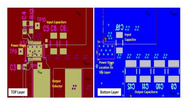
Figure 17. Recommended PCB Layout (Top Down View)
