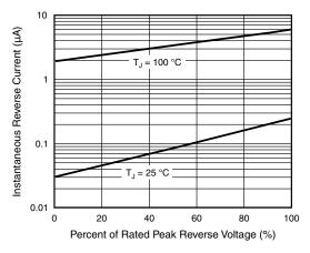
Fig. 5 - Typical Reverse Leakage Characteristics Per Diode
