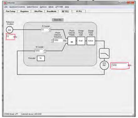
7. To program the settings into the device, Click "Keyboard Controls" → "Load Device", or Press CTRL + L
