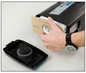
Figure 5: Removing and Changing the Filter
