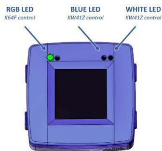
Figure 210. USB Programming LED
