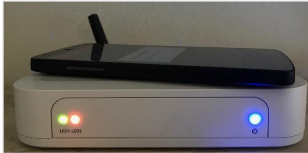
Figure 139. Gateway connected to the Cloud over WiFi
