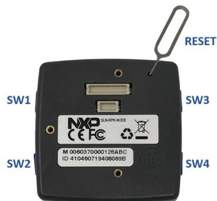
Figure 160. Bootloader push buttons
