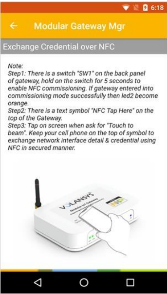
Figure 133. WiFi Provisioning over NFC
