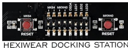
Figure 110. Docking Station Jumper Switch configuration to debug KW41Z
