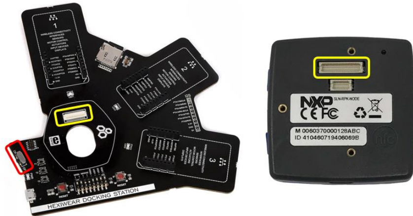
Figure 108. Docking station connector
