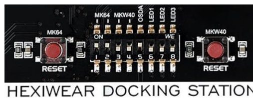
Figure 109. Docking Station Jumper Switch configuration to debug K64F
