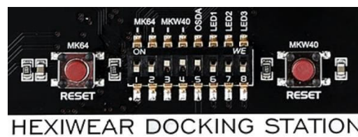
Figure 68. Docking Station Jumper Switch configuration to debug KW41Z
