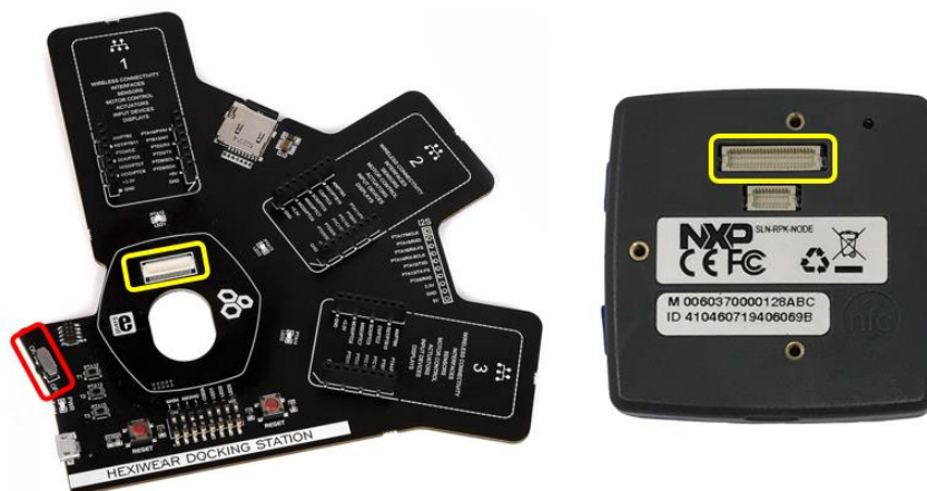
Figure 171. Docking station connector
