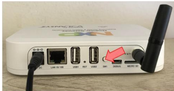
Figure 134. Initiate Gateway Commissioning
