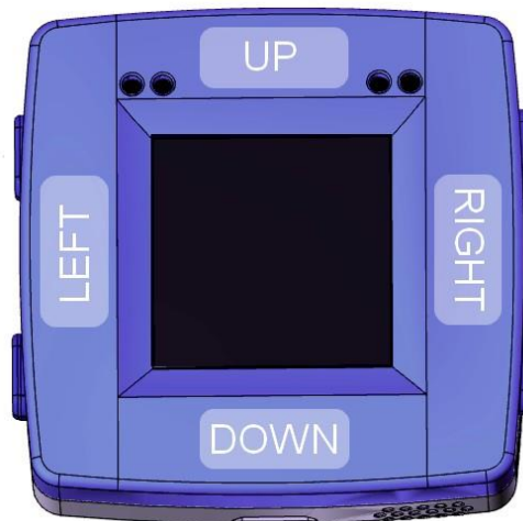
Figure 100. Touch electrodes location
