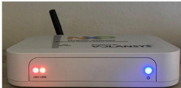
Figure 135. LED for Gateway Commissioning
