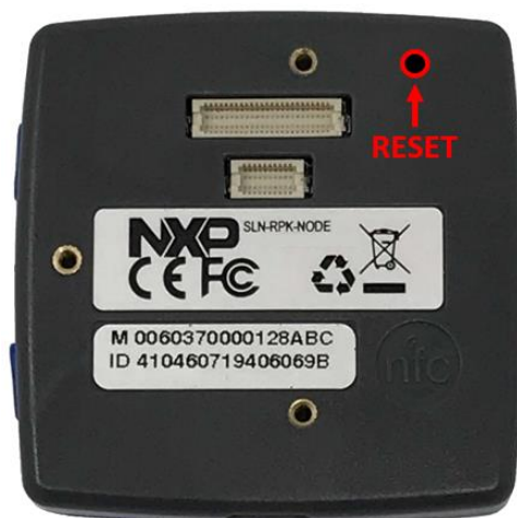
Figure 98. Rear view, Reset button location
