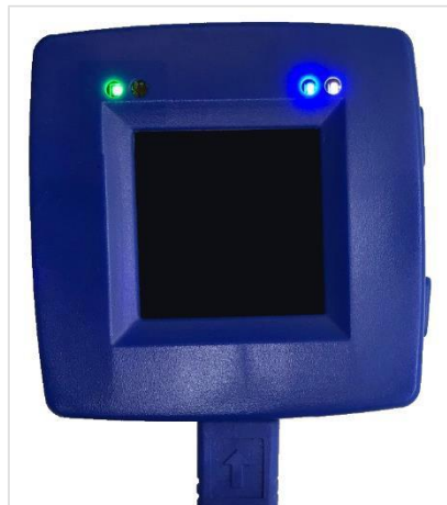
Figure 5. Bootloader Flash LEDs
