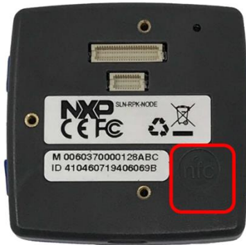
Figure 93. Rear view, NFC antenna location
