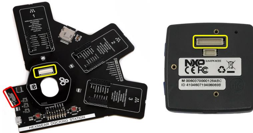
Figure 66. Docking station connector
