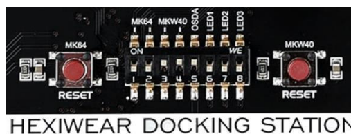
Figure 110. Docking Station Jumper Switch configuration to debug KW41Z
