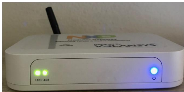
Figure 123. Gateway connected to Cloud over Ethernet
