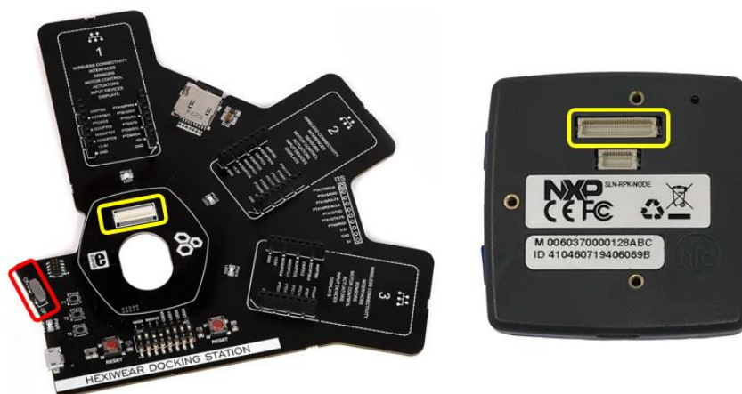
Figure 182. Docking station connector
