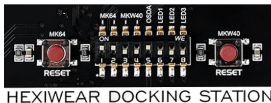
Figure 172. Docking Station Jumper Switch configuration to debug K64F
