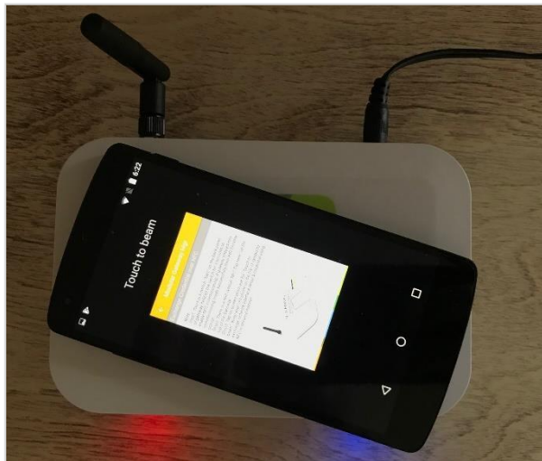
Figure 136. Phone positioning for NFC Commissioning
