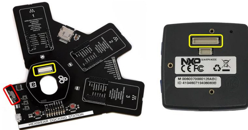
Figure 108. Docking station connector
