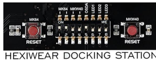
Figure 67. Docking Station Jumper Switch configuration to debug K64F
