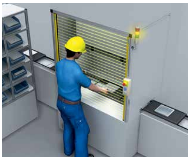
Single break PSDI mode on an automatic assembly system with a safety light curtain. During loading, the tool is in the open position. After the operator leaves the protective field, the assembly cycle begins.
