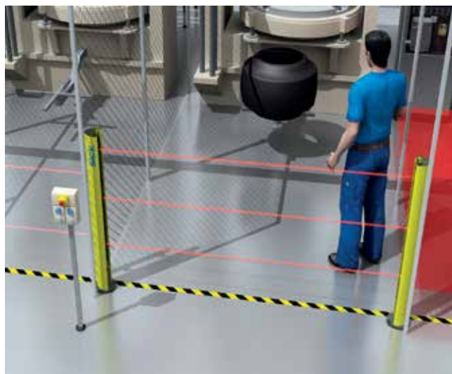
Access protection with a multiple light beam safety device
