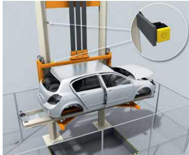
Safe position monitoring for a lift on an automobile production line
