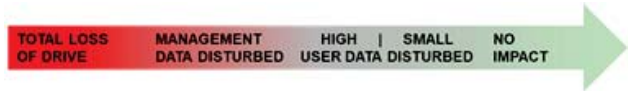
Figure 4-2: Consequences of a Sudden Power Failure (SPF)
