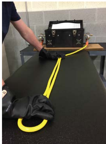
5. Grounding cable sets are tested to ASTM standard F2249-03. Current is applied on GT400HDXL Tester and the voltage drop measured.
