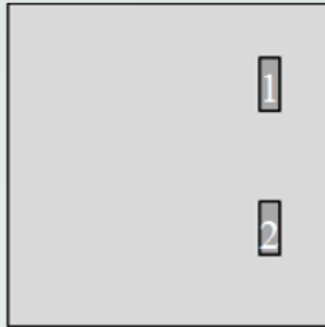
Figure 4. Representation of preform placement on QFN thermal pads. Square represents the entire 7.75 mm square thermal pad.
