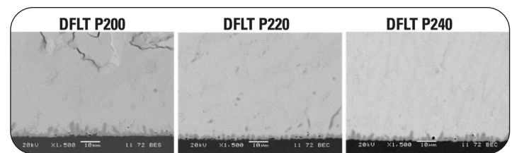
Figure 13. Interfacial IMC morphology at the PCB side with different reflow profiles.
