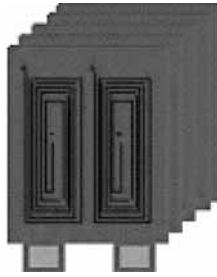
Figure 43: PRiME™ sensor multi-layers printed wiring board
