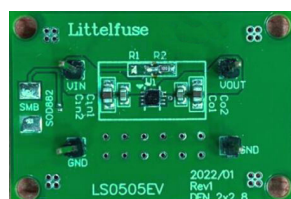
Figure 4. LS0505EVD22 EV. Board 5V, 5A with 30Vmax & OVP / OCP
