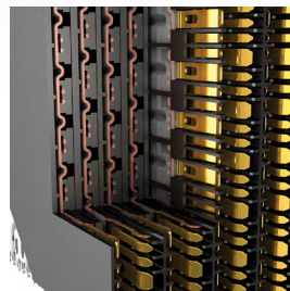
Staggered differential pair design
