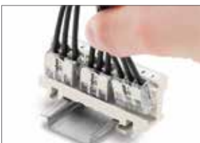
Install connectors into the mounting carrier
