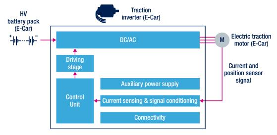
Tab. 3 - ST's products mapping for Traction Inverter
