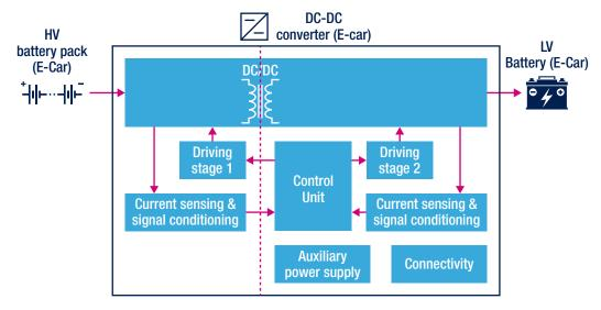
Tab. 4 - ST's products mapping for DC-DC Converter
