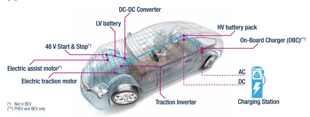
The Electric vehicles are classified by how electricity is used to power the vehicle:
