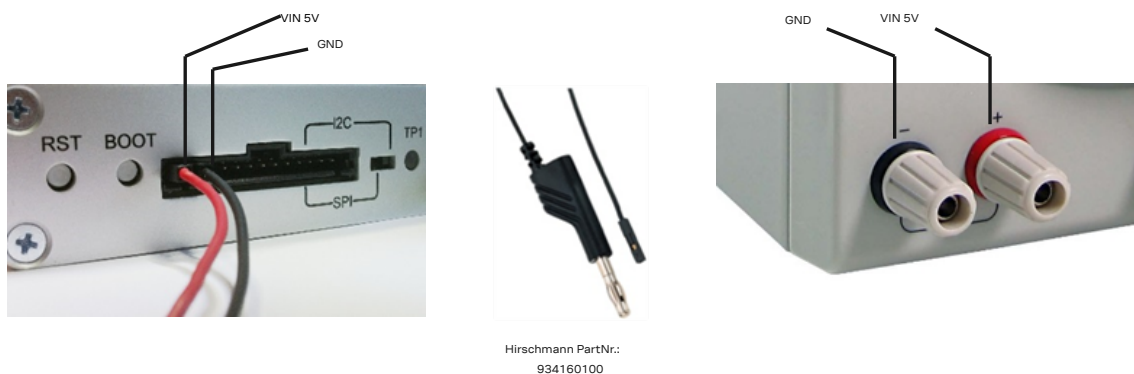
Figure 3: EVK-X20P 5.0 V DC power supply example
