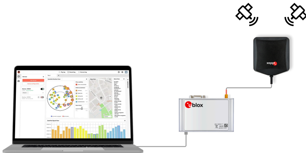
Figure 1: Connecting the EVK-X20P unit for power supply and communication
