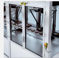
Access guarding on safety gates
