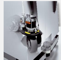
Simple steering angle detection for AGVs
