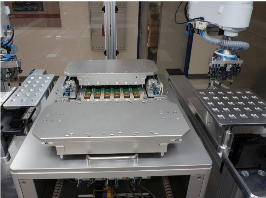
Figure 11: Automatic test equipment for module test
