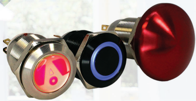
AH Series 19mm IP67 Sealing Degree Momentary Panel Mount 1A@24VDC / 125VAC, 0.5A@250VAC
