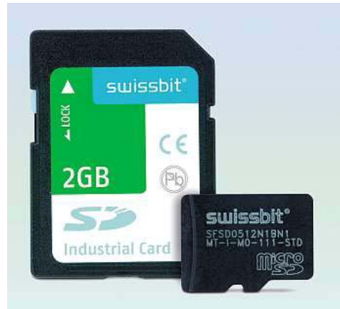
Image 2: Swissbit memory solutions such as these SD cards come with a 'fixed bill of material' – all products are structurally identical with the sample and hence 100% identical between themselves in all deliveries. (image: Swissbit)
