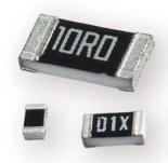
Yageo's thin film resistor RT series is a perfect solution for applications with high precision and high stability requirements. In thin film resistors, sputtering technology is used to form a nichrome (NiCr) resistive layer on the ceramic substrate. Compared to the printing process of thick film resistors, the metal resistive layer deposited by sputtering technology allows thin film
