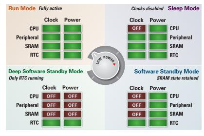
> The RX Series has four power modes to manage precious battery energy consumption without compromising performance
