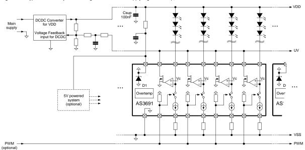
Figure 16 - Typical AS3691 system for single color leds and supply regulation loop; serveral AS3691 can be cascaded
