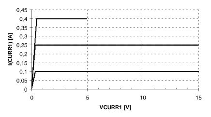
Figure 6 - Output Current versus Voltage on Current Source - Low Current Range
