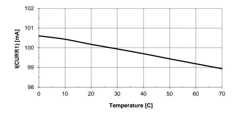
Figure 8 – Output Currnent versus Temperature, V(CURR1) = 2.0V, Ri1 = 2.5Ω (Note: temperature coefficient of Ri1 = -200ppm/°C)
