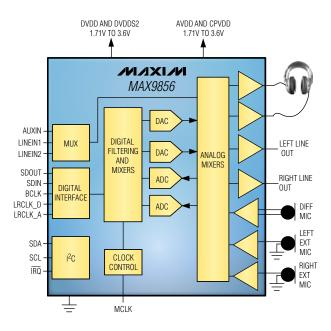
Simplified block diagram of the MAX9856 stereo audio codec.
