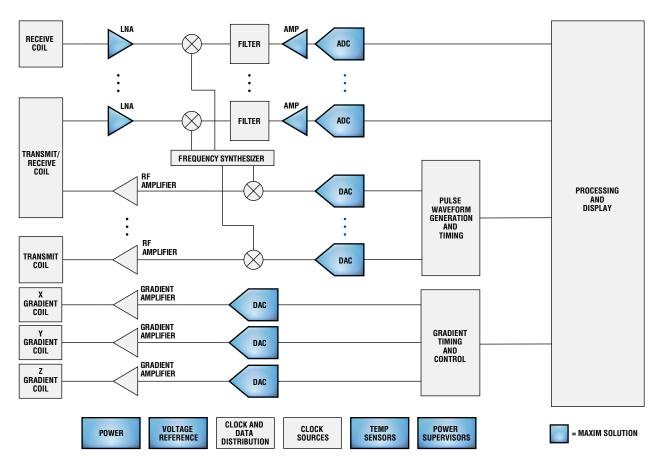
Block diagram of an MRI imaging system. For a list of Maxim's recommended MRI solutions, please go to: www.maxim-ic.com/mri.
