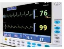
Patient monitor showing ECG and pulse oximetry readings.
