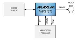
Block diagram for the MAX11811 in a haptic touch-screen application.
