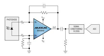
Typical operating circuit for the MAX9945 in a photodiode application.
