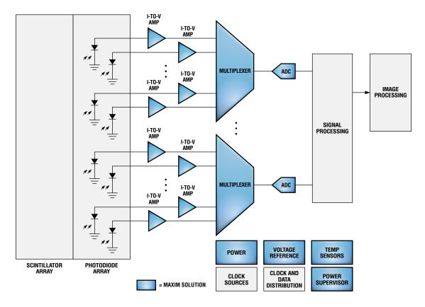
Block diagram of a CT imaging system. For a list of Maxim's recommended CT imaging solutions, please go to: www.maxim-ic.com/ct.
