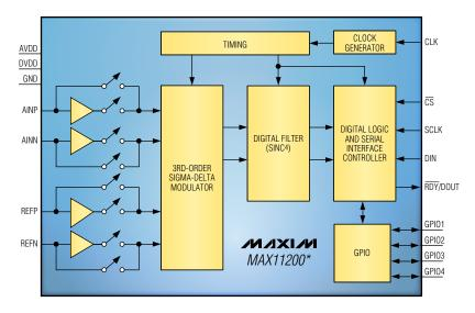
The MAX11200's integrated GPIOs allow control of an external 16-channel mux without needing additional isolation components.
