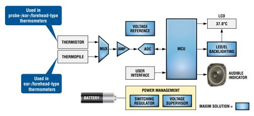
Functional block diagram of a digital thermometer. For a list of Maxim's recommended solutions for digital thermometer designs, please go to: www.maxim-ic.com/thermometer.
