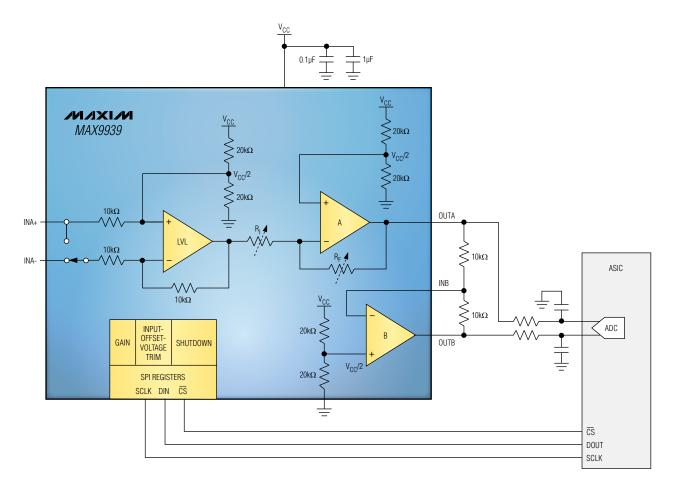
Typical operating circuit for the MAX9939 driving an ADC with a differential input.
