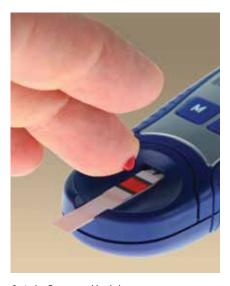
Optical-reflectometry blood glucose meter
