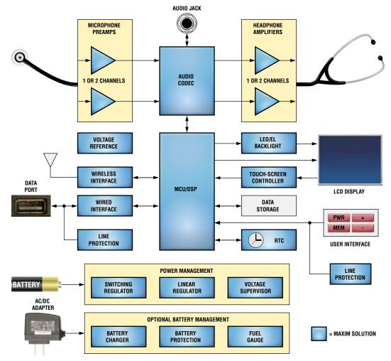
Functional block diagram of a digital stethoscope. For a list of Maxim's recommended digital-stethoscope solutions, please go to: www.maxim-ic.com/stethoscope.
