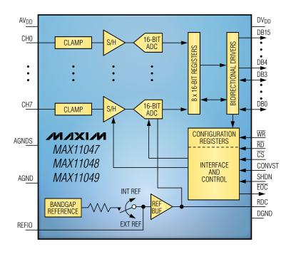
Block diagram of the MAX11047/MAX11048/MAX11049 ADCs.
