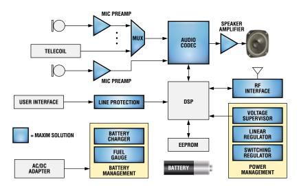
Digital hearing aid functional block diagram. For a list of Maxim's recommended solutions for hearing aid designs, please go to: www.maxim-ic.com/hearing.
