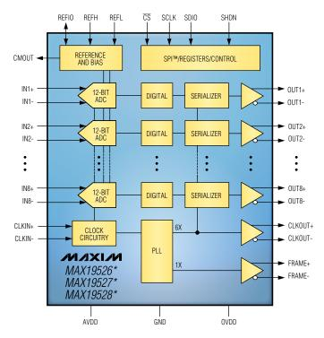
Block diagram of the MAX19526/MAX19527/MAX19528.
