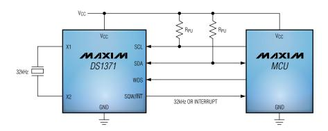
Typical application circuit for the DS1371 shows how the device drives the clock signal to the microcontroller through its square-wave output.
