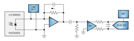
Figure 2. Simplified photodiode receive path circuit.
