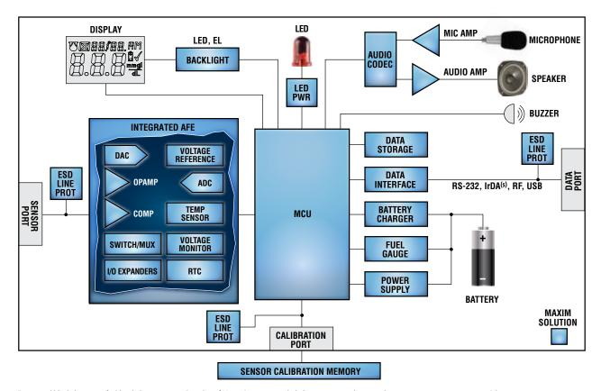
$Functional \ block\ diagram\ of\ a\ blood\ glucose\ meter.\ For\ a\ list\ of\ Maxim's\ recommended\ glucose-meter\ solutions,\ please\ go\ to: \underline{www.maxim-ic.com/glucose}.$
