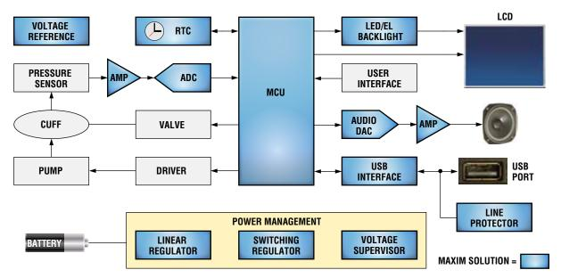
Functional block diagram of a blood pressure monitor that includes an advanced voice indicator. For a list of Maxim's recommended solutions for blood pressure monitor designs, please go to: www.maxim-ic.com/bloodpressure.
