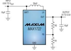
MAX1722 adjustable output voltage circuit
