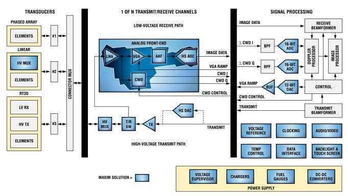
Functional block diagram of an ultrasound imaging system. For a list of Maxim's recommended ultrasound solutions, please go to: www.maxim-ic.com/ultrasound.
