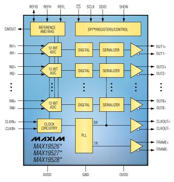
Typical operating circuit for the MAX19526/MAX19527/MAX19528.
