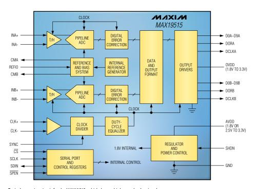
Typical operating circuit for the MAX19515, which detects high-speed pulse signals.
