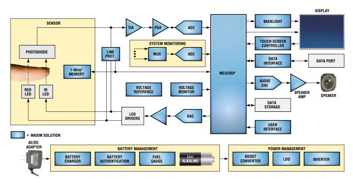
Functional block diagram of a pulse oximeter. For a list of Maxim's recommended solutions for pulse oximeters, please go to: www.maxim-ic.com/pulseox.
