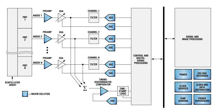
Block diagram of a PET system. This diagram shows one of multiple receiver groups that share a common time discriminator. For a list of Maxim's recommended PET solutions, please go to: www.maxim-ic.com/pet.
