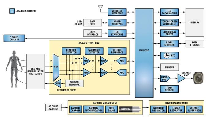
Full-featured ECG functional block diagram. For a list of Maxim's recommended solutions for an ECG design, please go to: www.maxim-ic.com/ECG.
