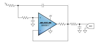
Typical application circuit: Sallen-Key active lowpass filter
