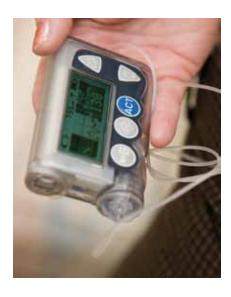
systems, a separate continuous monitor with a radio transmitter measures and reports blood glucose levels to a sensor-enabled pump. The pump, in turn, displays trend information with graphical charting of glucose history to aid insulin dosage calculations.
