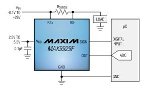
Typical operating circuit for the MAX9928F/MAX9929F.
