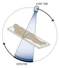
The patient is exposed to a fan-shaped x-ray beam, and the projected image is detected on a thin, semicircular digital x-ray detector.
