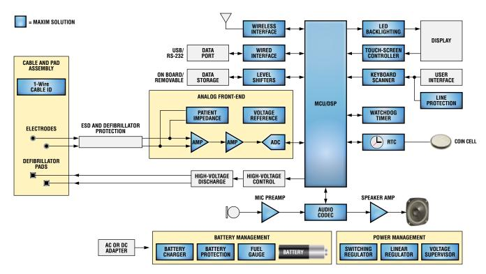
Functional block diagram for an AED device. For a list of Maxim's recommended solutions for an AED design, please go to: www.maxim-ic.com/ECG.
