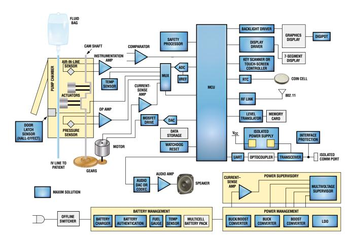
Functional block diagram of an infusion pump. For a list of Maxim's recommended solutions for infusion pumps, please visit: www.maxim-ic.com/infusion.
