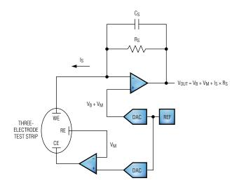
Figure 2. Electrochemical test strip in a counter configuration.
