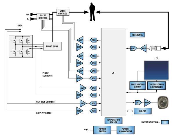
Functional block diagram of a ventilator system. For a list of Maxim's recommended solutions for ventilator designs, please go to www.maxim-ic.com/ventilator.
