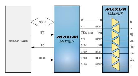
Typical operating circuit for the MAX3107 in an RS-232 application.
