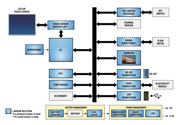
System block diagram of a desktop spirometer. For a list of Maxim's recommended solutions for spirometers, please visit: www.maxim-ic.com/spirometer.
