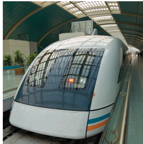
Figure 11. Maglev train driven by a linear motor.
