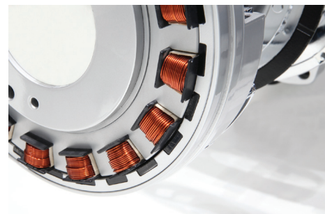
Figure 3. Disassembled outrunner BLDC motor. Fixed armature carries the stator windings. The rotor carries the permanent magnets.
